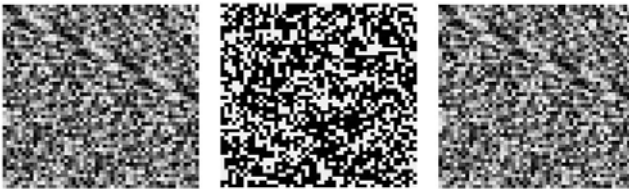
Fig. 9.9 In Example (9.30), the left is a 50 \times 51 sized image of the original image a_\sigma for a given 2-dimensional commutative linear representation system \sigma , the middle is added noises. The right is a 50 \times 51 sized image which displays the original image and added noise.
